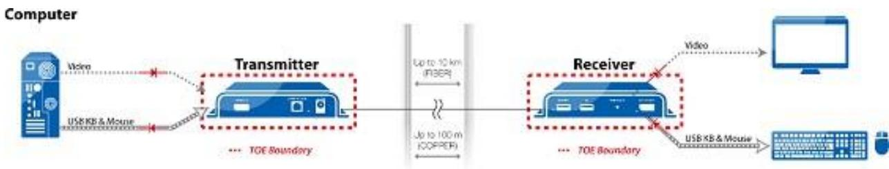
Figure 3: Isolator Evaluation Configuration
